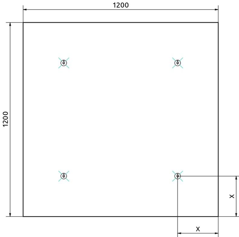
Distance from the edge of the Wall Absorber (X) 100–250mm
