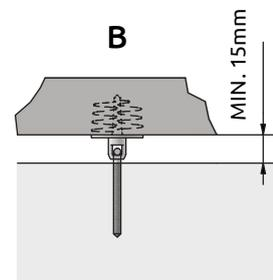
**Note:** The product is not secured against lifting nor protected against impact resistance, to secure the product, install it first and use a simple angle on top of the edge to prevent lifting.
