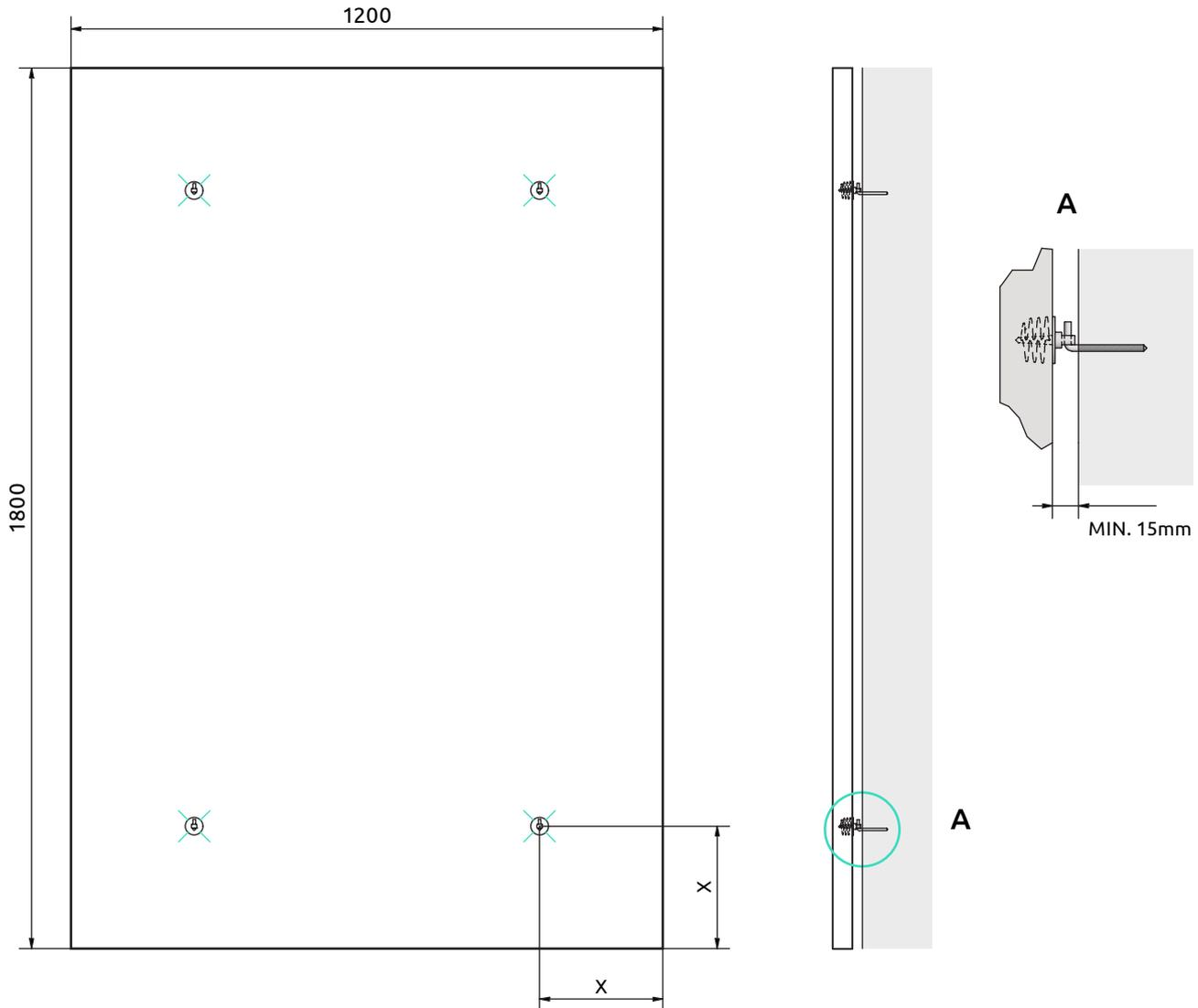
Distance from the edge of the Wall Absorber (X) 100–250mm
