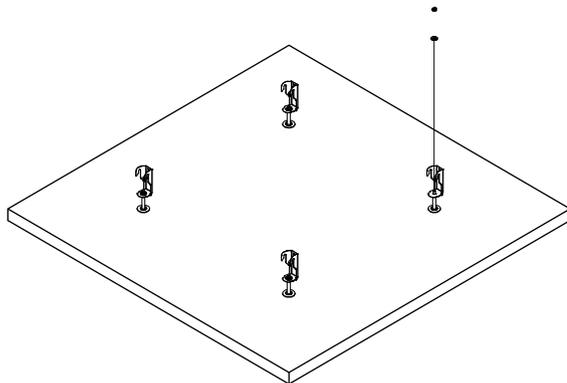
4. Place washer over the runner to anchor hanger (panel bracket), locating over the height adjustment screw thread
