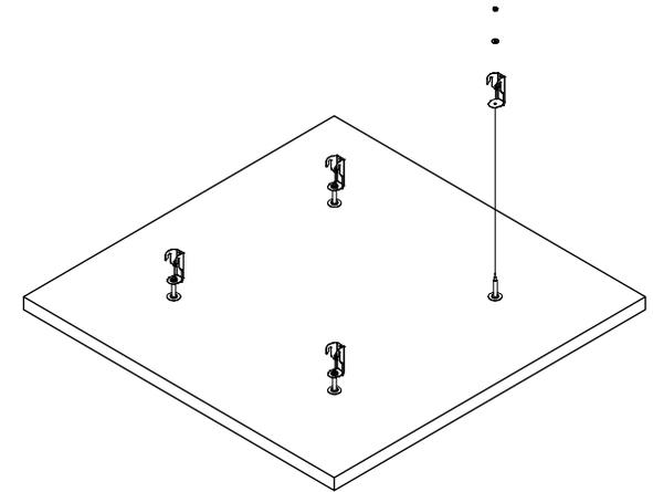
3. Place the runner to anchor hanger (panel bracket) in place on top of the height adjustment rod in the correct orientation as required for the assembly arrangement
