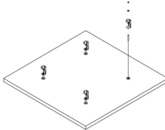
2. Locate correct height adjustment rod for assembly and place through washer and tighten into anchor screw thread
