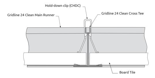
In case of high air pressure from below, hold-down clips need to be used to avoid uplift of tiles and to provide airtightness.
