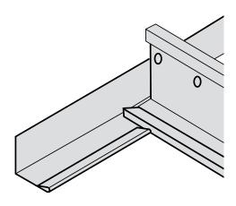
Where the grid is laid on top of the perimeter trim, the gasket of the perimeter trim needs to be cut and removed.
