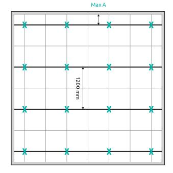
\*For alternative hanger and main runner spacing, please contact ITS on 0800 371 849
