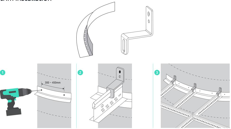
\*Tighter radii will require smaller fixing centres. First fixings max. 50mm from ends of trim
