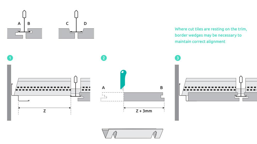
\*Spacer bars are recommended at the perimeters of all installations to maintain proper tile alignment
