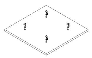
6. Final assembly of height adjustment rods
