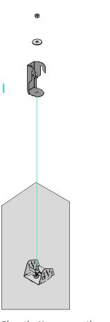
Place the Hanger over the screw thread and align the hanger to the direction you need the canopy to be angled
