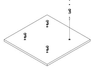
2. Locate correct height adjustment rod for assembly and place through washer and tighten into anchor screw thread
