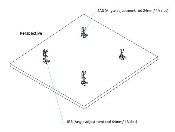
1BS (Angle adjustment rod 64mm/ 1B slot)
