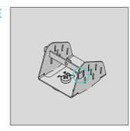
Tab bent and secured
