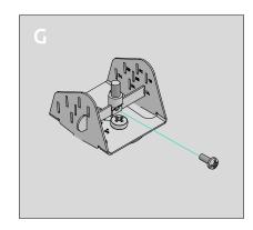
Use the M4 screw to secure rod in place
