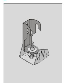
The assembly for the 1st angled bracket is complete, repeat as required for the front of the canopy
