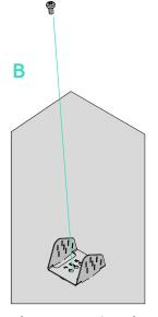
Place M6 scew into the bracket hole and anchor to secure
