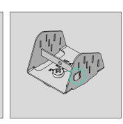
Tab bent and secured
