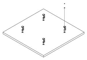
Place washer over the runner to anchor hanger (panel bracket), locating over the height adjustment screw thread
