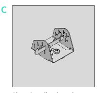
Place the splint through slot 1B for a 5 degree angle, referring to the engraving on the bracket for the required location
