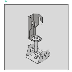
The assembly for the 2nd angled bracket is complete, repeat as required for the canopy
