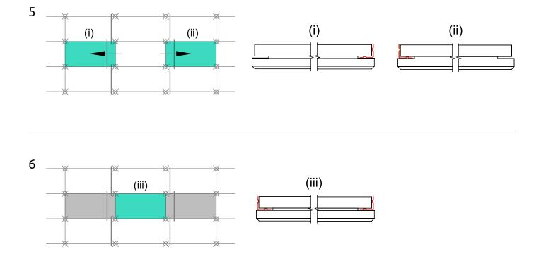
\*If preferred, L-Bars can be inserted into tiles (i), (ii) before they are installed.
