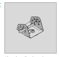
Place the splint through slot 1B for a 5 degree angle, referring to the engraving on the bracket for the required location
