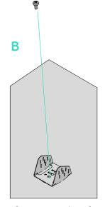
Place M6 scew into the bracket hole and anchor to secure
