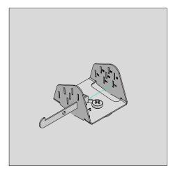
Place the splint through slot 1A for a 5 degree angle, referring to the engraving on the bracket for the required location
