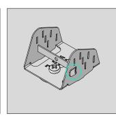
Tab bent and secured
