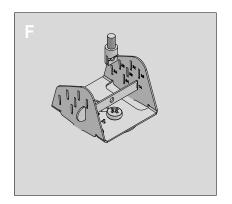
Locate associated rod which matches slot engraving align holes in the rod and splint
