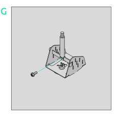
Use the M4 screw to secure rod in place
