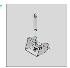
Locate associated rod which matches slot engraving align holes in the rod and splint
