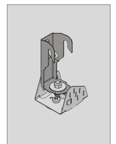
The assembly for the 1st angled bracket is complete, repeat as required for the front of the canopy
