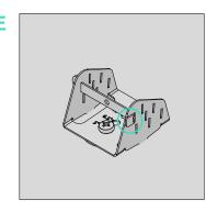
Tab bent and secured
