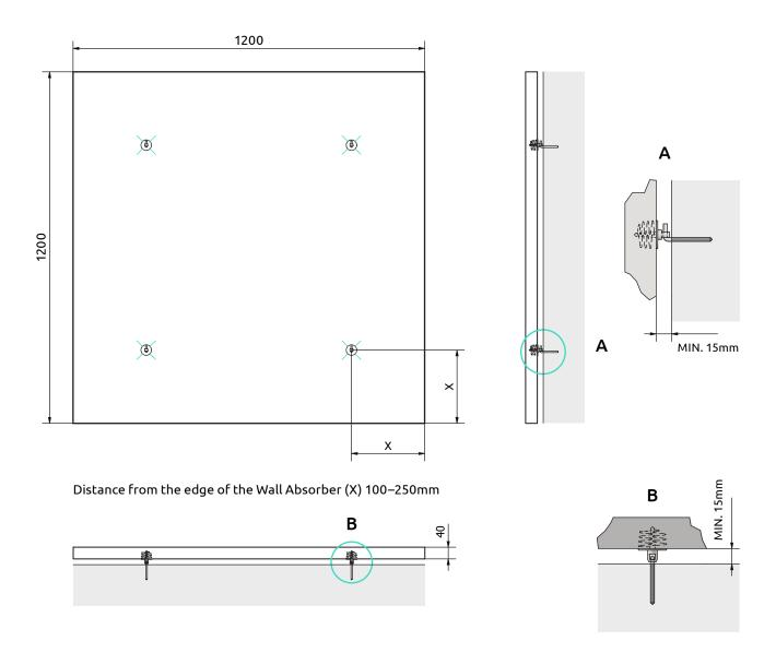
**Note:** The product is not secured against lifting nor protected against impact resistance, to secure the product, install it first and use a simple angle on top of the edge to prevent lifting.
