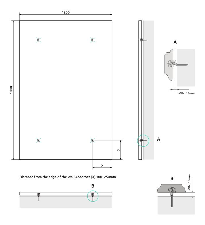
**Note:** The product is not secured against lifting nor protected against impact resistance, to secure the product, install it first and use a simple angle on top of the edge to prevent lifting.
