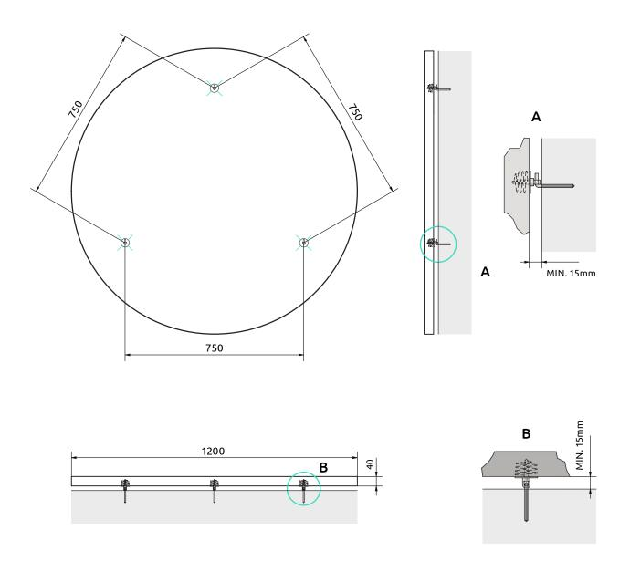
**Note:** The product is not secured against lifting nor protected against impact resistance, to secure the product, install it first and use a simple angle on top of the edge to prevent lifting.
